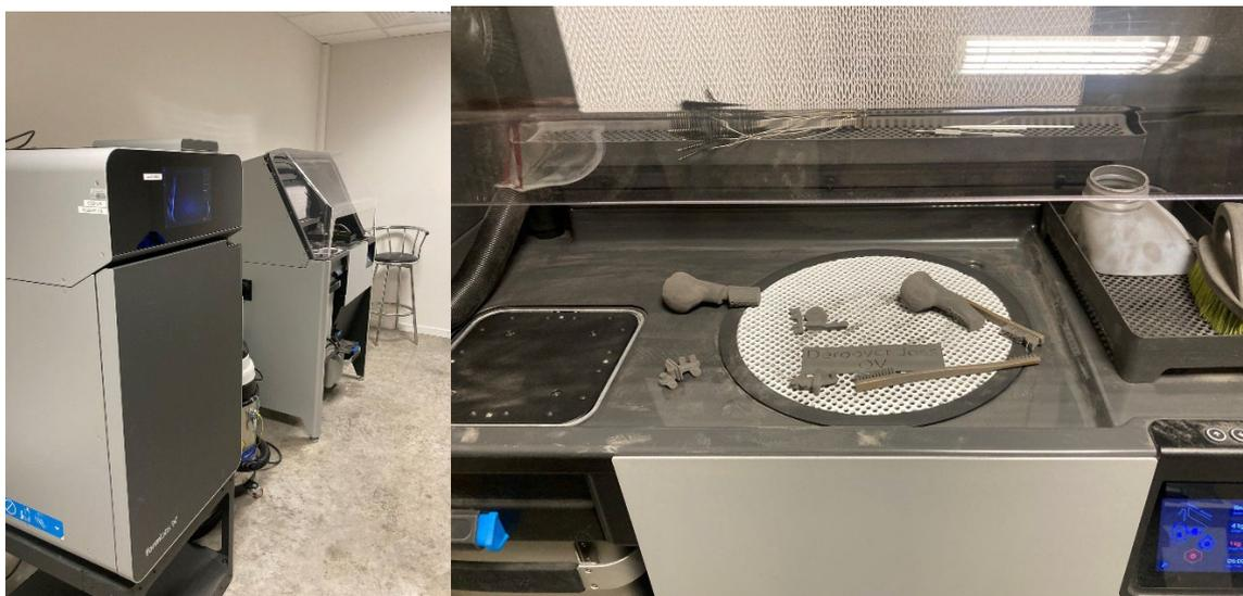
*Figure 13. a) 3D printer b) Printed models and guides for intra operative use.*
